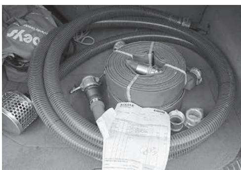
Fire-pump accessories (suction hose and strainer, camlocks, discharge hoses, couplings, and hose nozzle) are stored with the TLA fire pump in the red wooden box on the fixed dock at the Headquarters Building. (photo by Rob Corcoran)
