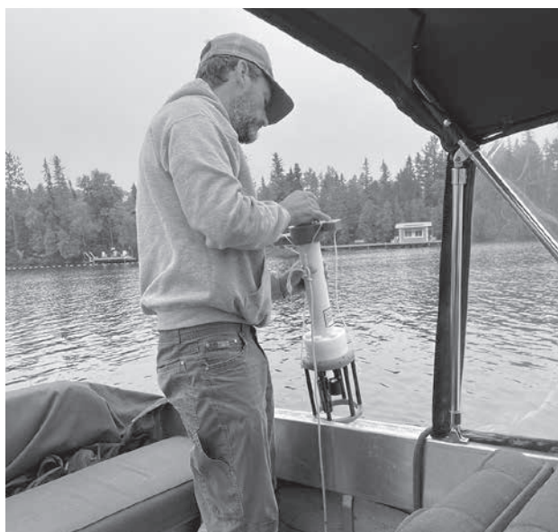
Dr. Murray Richardson Drops a Sonde (an instrument probe that transmits information about water-quality characteristics) into the NE Arm (photo by Tim Richardson)
