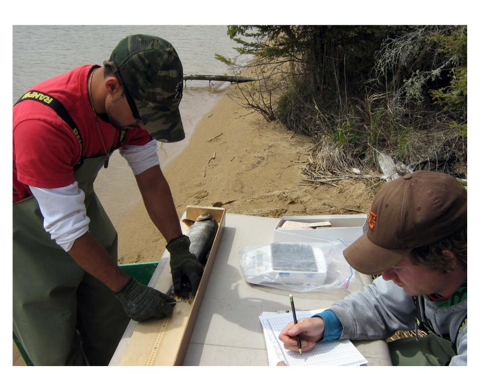
A crew measuring and recording fish length and weight (as well as other characteristics not shown).
