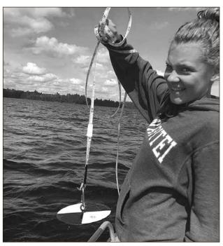
Lauren Richardson With a Secchi Disk [device to determine the transparency of water by measuring the depth at which the disk ceases to be visible from the surface] (photo by Louise Richardson)
